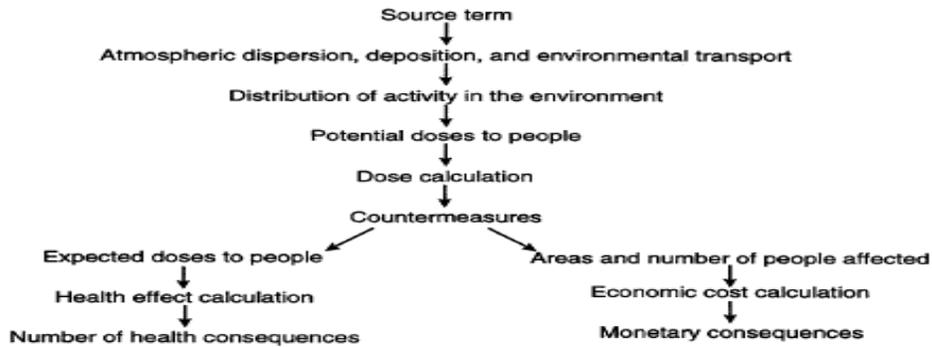
Figure 1. Scope of Accident Consequence Codes
