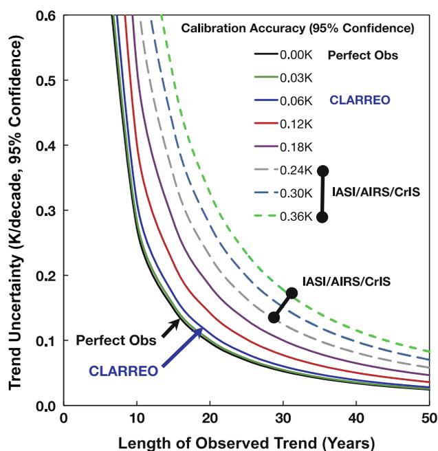
**Fig. 2** The relationship between global average temperature trend accuracy, length of a climate record, and satellite sensor calibration absolute accuracy. Current satellite observations include IASI/AIRS/CriS weather sensors. CLARREO represents a future higher accuracy sensor following the NRC decadal survey recommendations (2007). From Wielicki et al. (2013)
